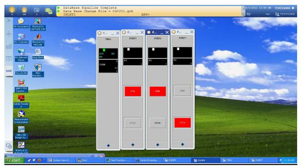
**THE FINAL PUMP (SPRAYING OF WATER) AUTOMATICALLY STARTS:** According to our logic, since both the weigh feeders start their movement, the output pump, **WATER SPRAYER** starts spraying the water.
